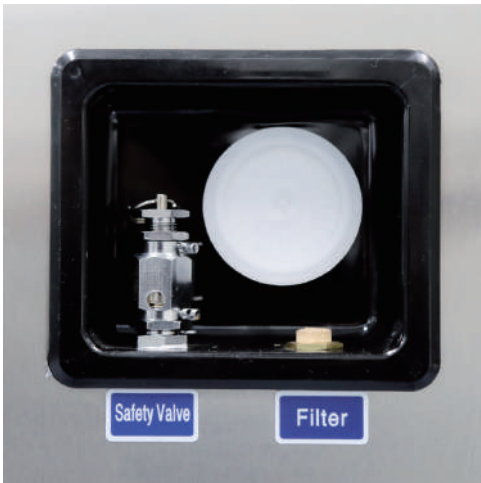
Air Filter → Prevention of backflow
